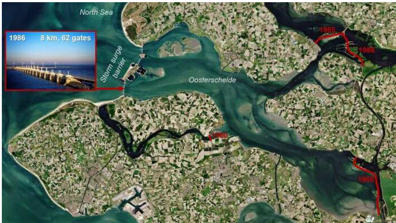
Overview of The Oosterschelde with its storm surge barrier and closure dams (indicated with the red lines, including years of completion). Satellite picture, credit: Copernicus Sentinel data (2020), processed by ESA, CC BY-SA 3.0 IGO.
